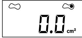
21. Repeat steps 9 and 10 for the first area of non-viable tissue. When processing is complete the unit will BEEP and display the non-viable tissue area in cm<sup>2</sup>.
