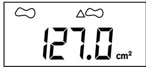
Touch each number in turn with the stylus, e.g. if the previous area was 127cm<sup>2</sup>, then enter '1', '2', '7', '0'. If an error is made, touch the 'C' button momentarily for each incorrect digit. Re-enter the correct digits.
